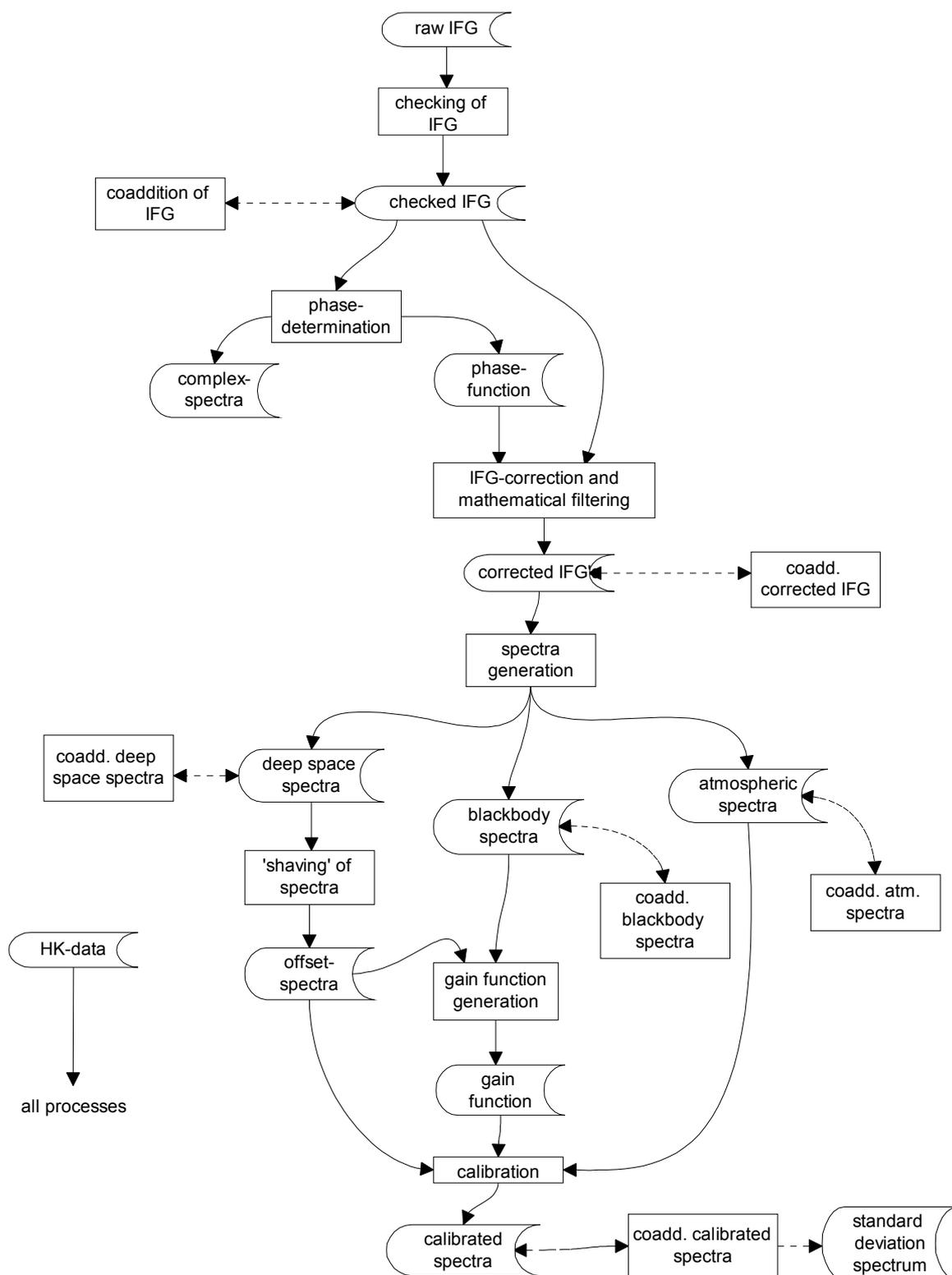
**fig. 2:** Dataflow diagram of the MIPAS-B2 data processing chain (apodisation is performed during every generation of a spectrum)
