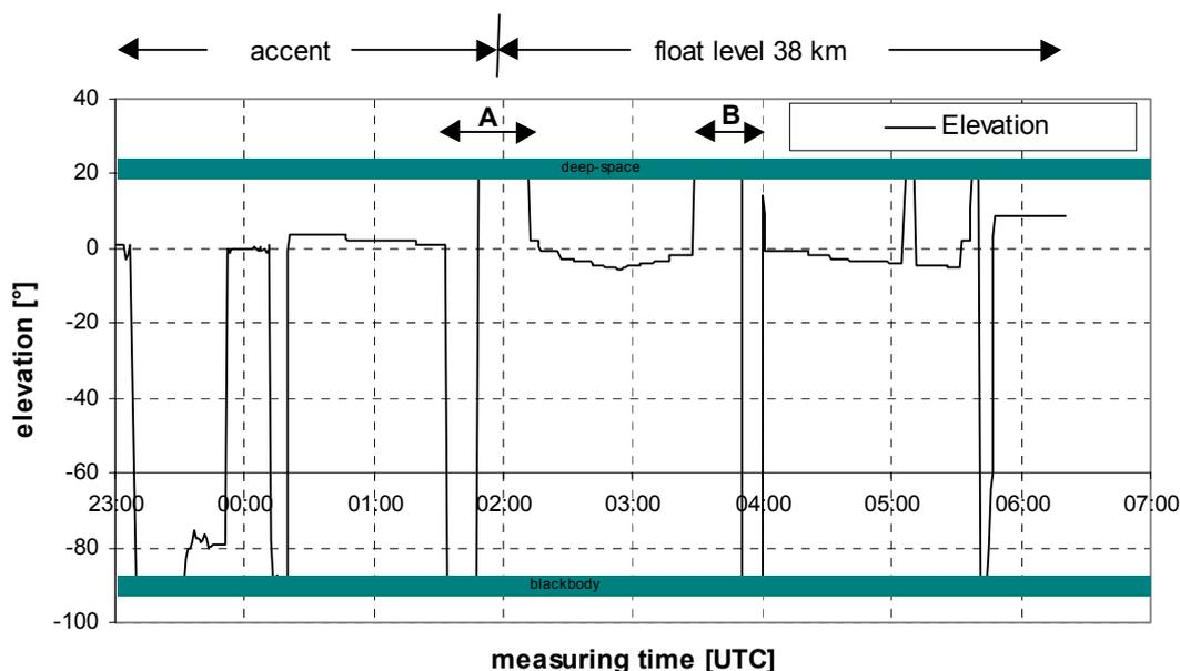
**fig. 1:** Measuring scenario of the MIPAS-B2 flight on 8.5.1998 at Aire sur l'Adour. The limb sequence is taken between the calibration cycles (A) and (B). The calibration cycles comprises each of a blackbody and deep-space measurements.
